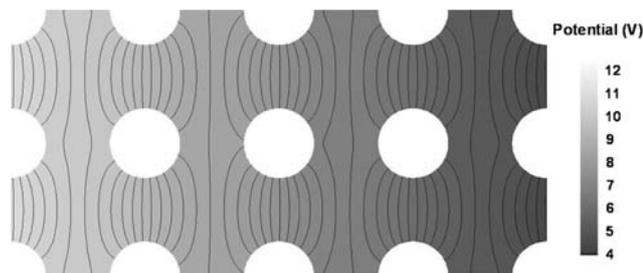
**Fig. 2** The distribution of electric potential in the microchannel for an external electric field of 25 V/mm. The curved lines are isopotential lines
