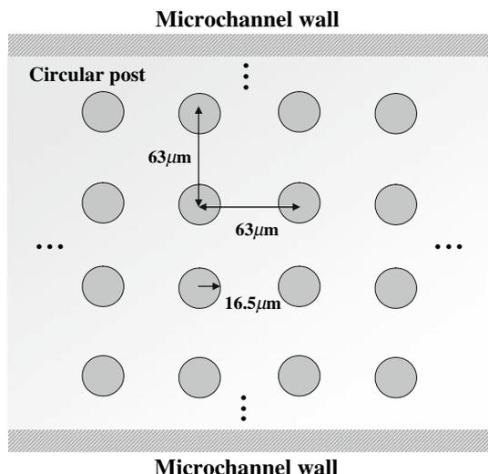
**Fig. 1** The geometry of the reference microchannel
