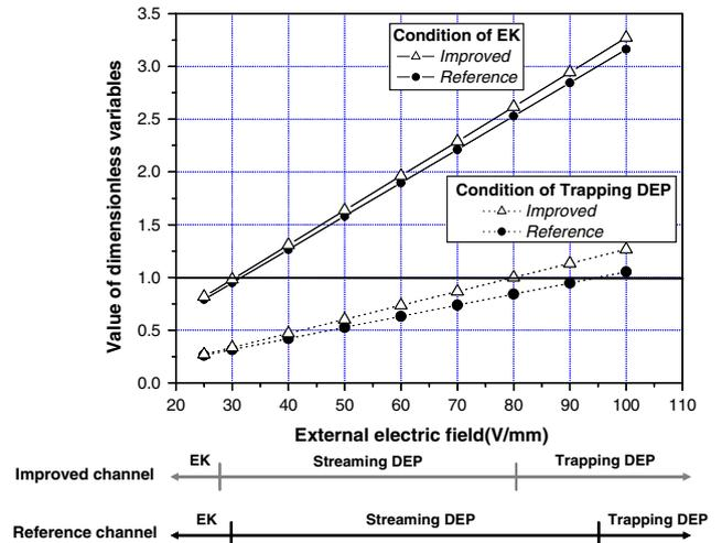
**Fig. 10** The variation of dimensionless variables for improved and reference microchannels with respect to the external electric field
