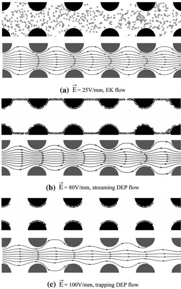
**Fig. 4** The three particle flow types driven by the external DC electric field. *Top figures* in **a–c** are obtained from Monte-Carlo simulations and the *bottoms* show the pathlines of particles
