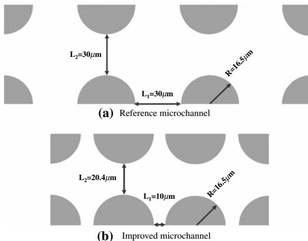
**Fig. 7** Comparison of the reference and improved microchannels. They are drawn to scale for convenient comparison. The values of  $L_2/(L_1 + 2R)$  remains the same between the two microchannels
