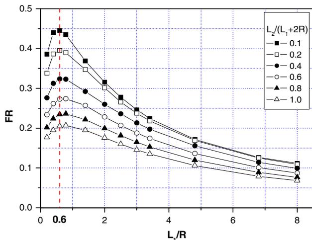
**Fig. 6** The variation of force ratio (FR) with respect to geometric parameters. The post radius is 16.5  $\mu\text{m}$
