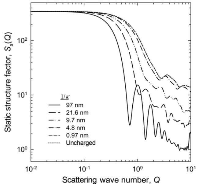
Fig. 6. Static structure factor  $S_s(\mathbf{Q})$  of the  $N_b = 25$  chains for different values of Debye screening thickness  $\kappa^{-1}$  corresponding to  $I = 0.01, 0.2, 1.0, 4.0,$  and  $100$  mM.
