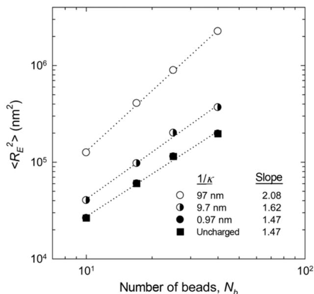
Fig. 3. The end-to-end distance versus the number of beads for different values of Debye screening thickness.  $\kappa^{-1}$  of 97, 9.7, and 0.97 nm corresponds to solution ionic concentration of 0.01, 1.0, 100 mM.
