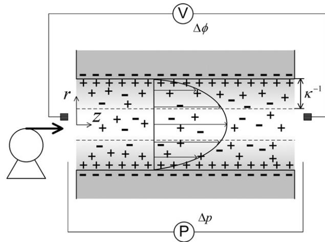
**Figure 1.** Schematic of electrokinetic streaming potential in a microfluidic channel.
