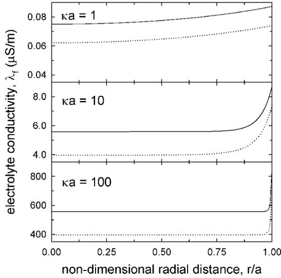
**Figure 3.** Fluid conductivity profiles for several dimensionless inverse EDL thicknesses for monovalent electrolytes of KCl (full) and LiClO<sub>4</sub> (dotted),  $\Psi_s = 1$ .
