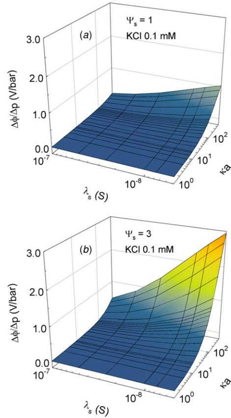
**Figure 6.** Effect of microchannel radius  $a$  on  $\Delta\phi/\Delta p$  with different surface conductivities  $\lambda_s$  for (a)  $\Psi_s = 1$  and (b)  $\Psi_s = 3$ , where  $\Delta p = 10$  bar and  $L = 10^{-2}$  m.
