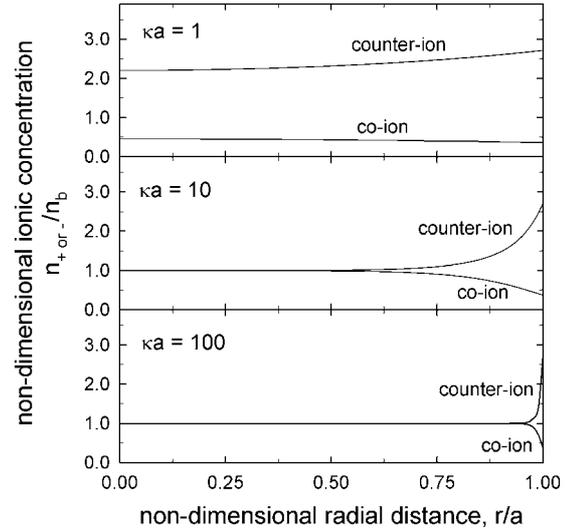
**Figure 2.** Number density profiles for co- and counter-ions in a microchannel for several dimensionless inverse EDL thicknesses,  $\Psi_s = 1$ .
