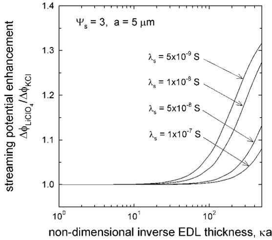
**Figure 5.** Effect of bulk electrolyte concentration on  $\Delta\phi_{\text{LiClO}_4}/\Delta\phi_{\text{KCl}}$  with different surface conductivities  $\lambda_s$ , where  $\Delta p = 10$  bar and  $L = 10^{-2}$  m.
