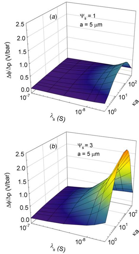
**Figure 4.** Effect of bulk concentration of KCl electrolyte on  $\Delta\phi/\Delta p$  with different surface conductivities  $\lambda_s$  for (a)  $\Psi_s = 1$  and (b)  $\Psi_s = 3$ , where  $\Delta p = 10$  bar and  $L = 10^{-2}$  m.
