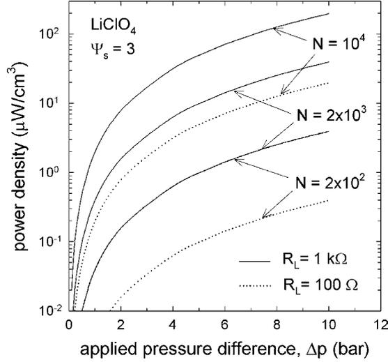
**Figure 8.** The predicted power density for  $\text{LiClO}_4$  electrolyte as a function of  $\Delta p$  with different external resistances and numbers of channels, where  $a = 5 \mu\text{m}$ ,  $\kappa a = 10$ ,  $L = 2 \times 10^{-3} \text{ m}$  and  $\lambda_s = 5 \times 10^{-9} \text{ S}$ .
