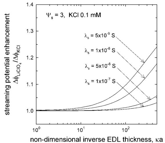
**Figure 7.** Effect of microchannel radius  $a$  on  $\Delta\phi_{\text{LiClO}_4}/\Delta\phi_{\text{KCl}}$  with different surface conductivities  $\lambda_s$ , where  $\Delta p = 10$  bar and  $L = 10^{-2}$  m.
