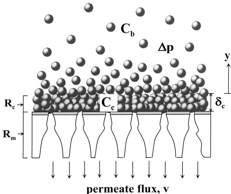
Fig. 1. Schematic diagram of dead-end filtration of colloidal suspension.
