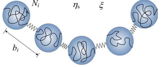
Fig. 1. (Color online) Illustration of the polyelectrolyte chain model with  $N$  segments and  $N - 1$  springs.
