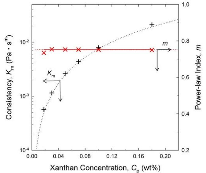
Fig. 4. (Color online) Dependence of the first normal stress difference parameters ( $K_m$  and  $m$ ) on the xanthan concentration  $C_p$  obtained by fitting for experimental data of Fig. 2(b). The dotted lines are the best fitting for  $K_m$  and  $m$ .
