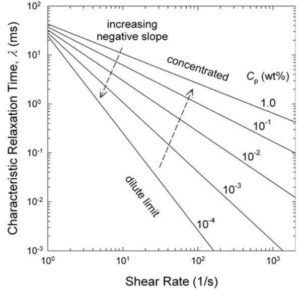
Fig. 6. Empirically determined characteristic relaxation time as functions of shear rate and xanthan concentration.
