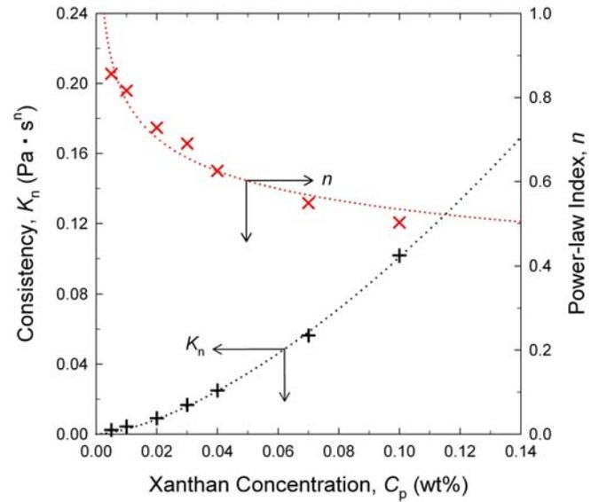
Fig. 3. (Color online) Dependence of the viscosity parameters ( $K_n$  and  $n$ ) on the xanthan concentration  $C_p$  obtained by fitting for experimental data of Fig. 2(a). The dotted lines are the best fitting for  $K_n$  and  $n$ .
