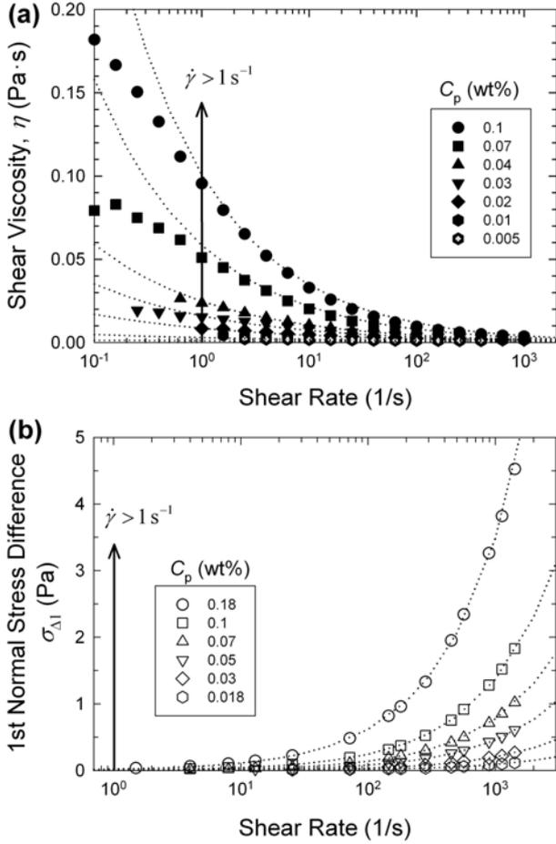
Fig. 5. Comparisons between experimental data and empirical correlations indicated by dotted curves for (a) shear viscosity and (b) first normal stress difference. Empirical curves are obtained by Eqs. (16) and (17), respectively.
