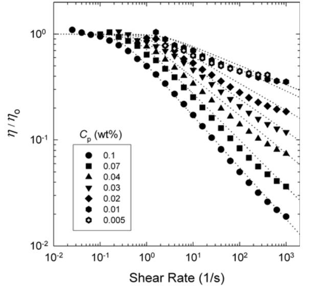
Fig. 7. Master plot of the shear viscosity after being normalized by  $\eta_0$  as a function of shear rate for different xanthan concentrations. The dotted curves are the best fitting on the basis of the Carreau A model.
