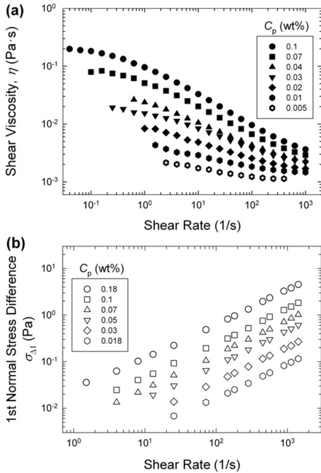
Fig. 2. Rheological data of (a) shear viscosity  $\eta$  and (b) first normal stress difference  $\sigma_{\Delta 1}$  as functions of shear rate  $\dot{\gamma}$  and xanthan polyelectrolyte concentration  $C_p$  at room temperature.
