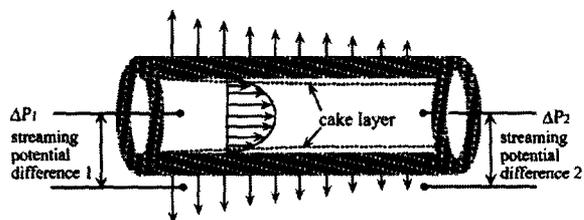
Fig. 1. Schematic of both local streaming potential differences and local pressure drops generated at inlet and outlet positions of a hollow-fiber membrane during colloid filtration.
