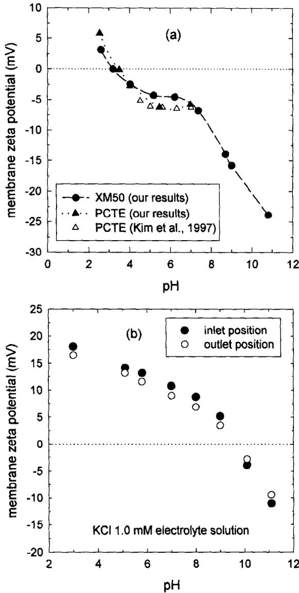
Fig. 3. The membrane zeta potential as a function of solution pH at 1.0 mM KCl concentration for flat-plate (a) and hollow fiber at inlet and outlet positions (b).
