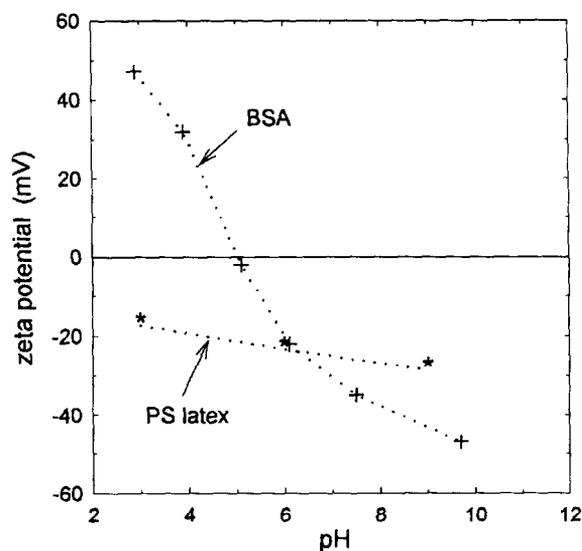
Fig. 2. The plots of zeta potential vs. pH for polystyrene latex and BSA protein with solution ionic strength of 1.0 mM KCl.
