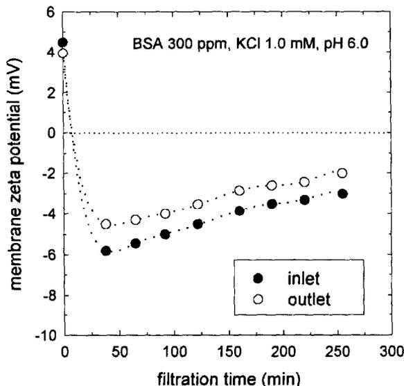
Fig. 5. Changes in axial position-dependent membrane zeta potential during the filtration of suspension with BSA 300 ppm. Experiments were performed with a PM100 hollow-fiber membrane at 0.2 atm of trans-membrane pressure.
