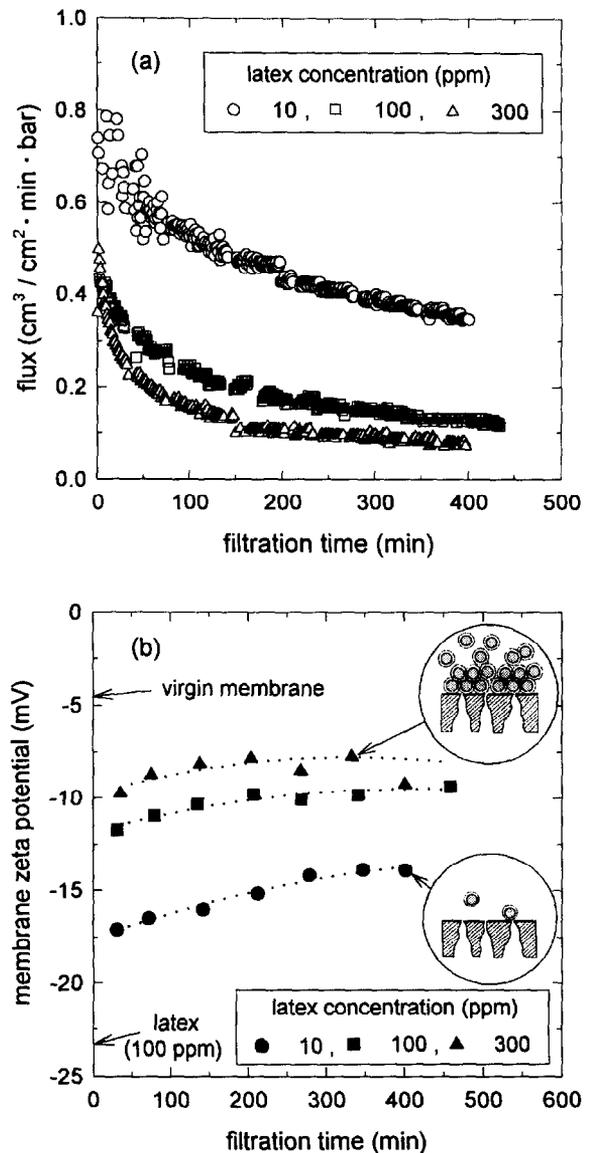
Fig. 4. Changes in the permeate flux (a) and membrane zeta potential (b) during the filtration as a function of latex concentration. Experiments were performed with an XM50 flat-plate membrane at 0.5 atm of transmembrane pressure, pH 6.0 and KCl 1.0 mM.
