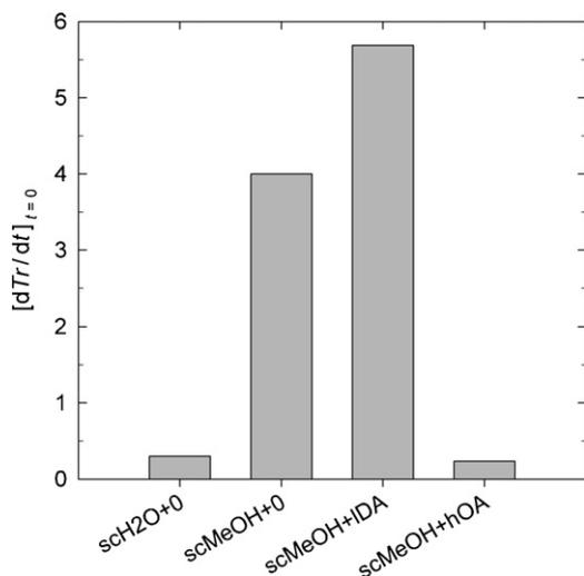
**Fig. 3.** Initial slopes of transmittance curves provided in Fig. 2 for the unmodified and the surface-modified CeO<sub>2</sub> nanoparticles.
