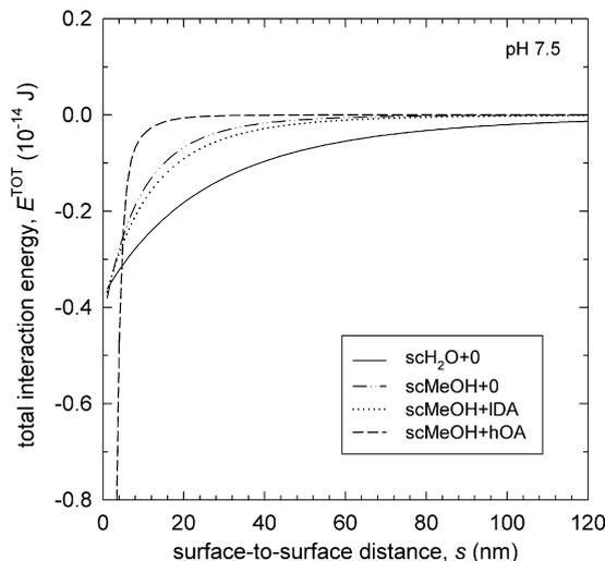
**Fig. 4.** Total interaction energy profiles for the unmodified and the surface-modified CeO<sub>2</sub> nanoparticles dispersed in ethylene glycol medium at pH 7.5. The nanoparticle concentration was 0.01 wt%.
