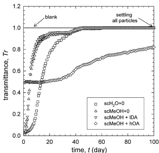
**Fig. 2.** UV transmittance of the unmodified and the surface-modified CeO<sub>2</sub> nanoparticles dispersed in ethylene glycol medium. The nanoparticle concentration was 0.01 wt%. The measurements were carried out at a wavelength of 400 nm.
