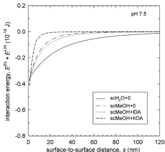
**Fig. 5.** Electrostatic and van der Waals interaction energy profiles for the unmodified and the surface-modified  $\text{CeO}_2$  nanoparticles dispersed in ethylene glycol medium at pH 7.5. The nanoparticle concentration was 0.01 wt%.
