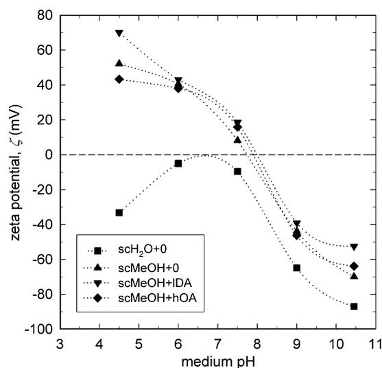
**Fig. 1.** Zeta potential values of the unmodified and the surface-modified CeO<sub>2</sub> nanoparticles dispersed in ethylene glycol medium at different pH values. The nanoparticle concentration was 0.01 wt%.
